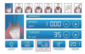
Touch the "Water volume" key on the screen to adjust. There are 6 water levels. The water level will change to the next level after each touch.
