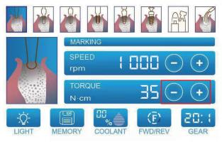
Touch the "Torque" (+, -) key to adjust maximum torque output of motor. The torque will change each time after touching the "Torque" key. Long press the "Torque" key to accelerate the change of torque setting value.
