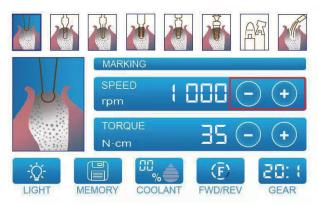
Touch the "Speed" (+, -) key to adjust motor speed. The speed will change each time after touching the "Speed" key. Long press the "Speed" key to accelerate the change of speed setting value.
