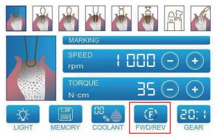
Touch the key shown above to change the rotating direction of motor.
