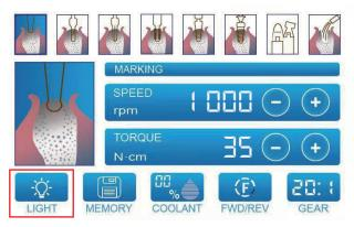
Touch the "LED" button to for setting to determine the on or off state of LED while stepping on foot pedal. The state of LED will change once after each touch. Only the device with LED owns this function.
