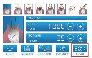
Adjust by pressing the "Speed Ratio" button to match the gear ratio of the handpiece to be used.
